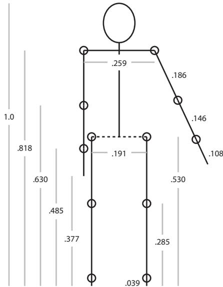
Figure 1. A sample of Drillis and Contini's proportionality constants [1].
